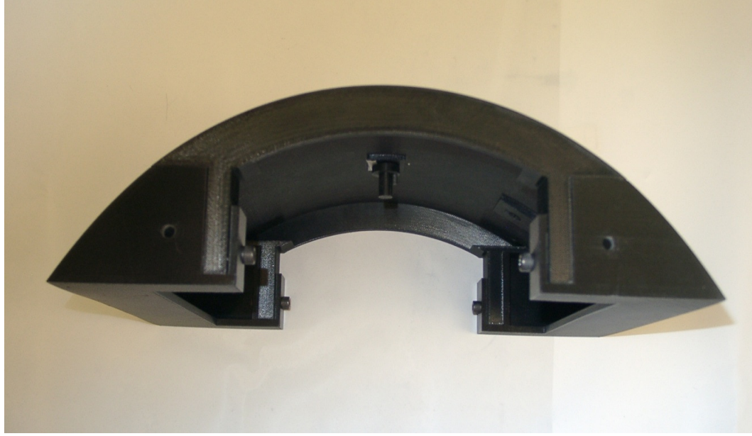
Figure 27: Tip for big (16" diameter) cylinder.
