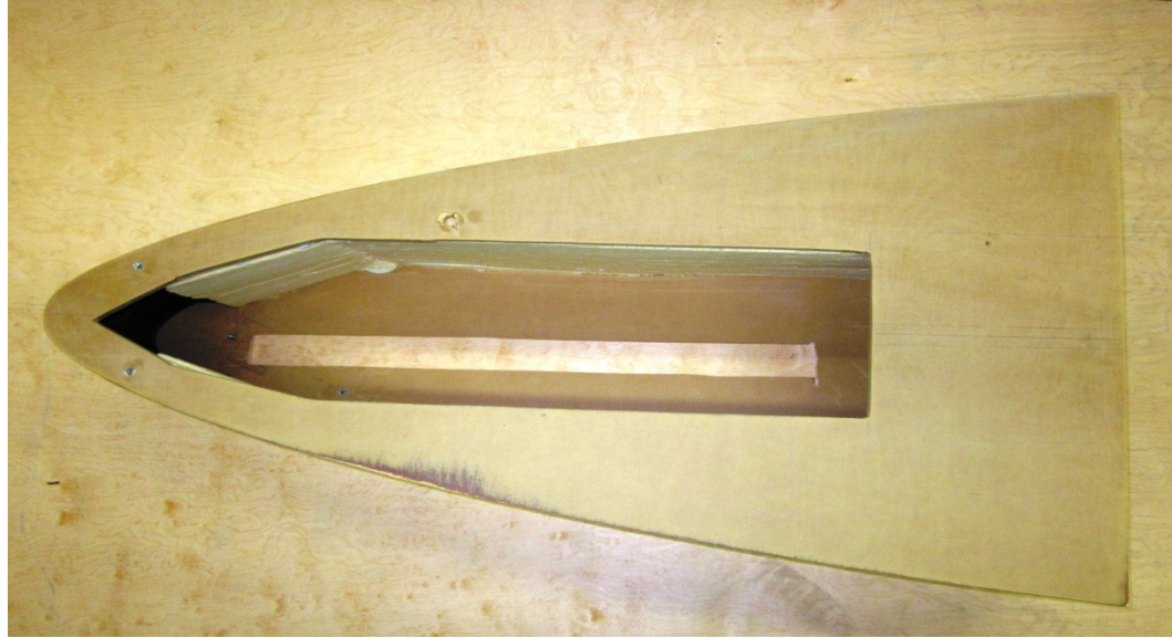
Figure 22: Top view of 4" diameter leading edge cylinder body.
