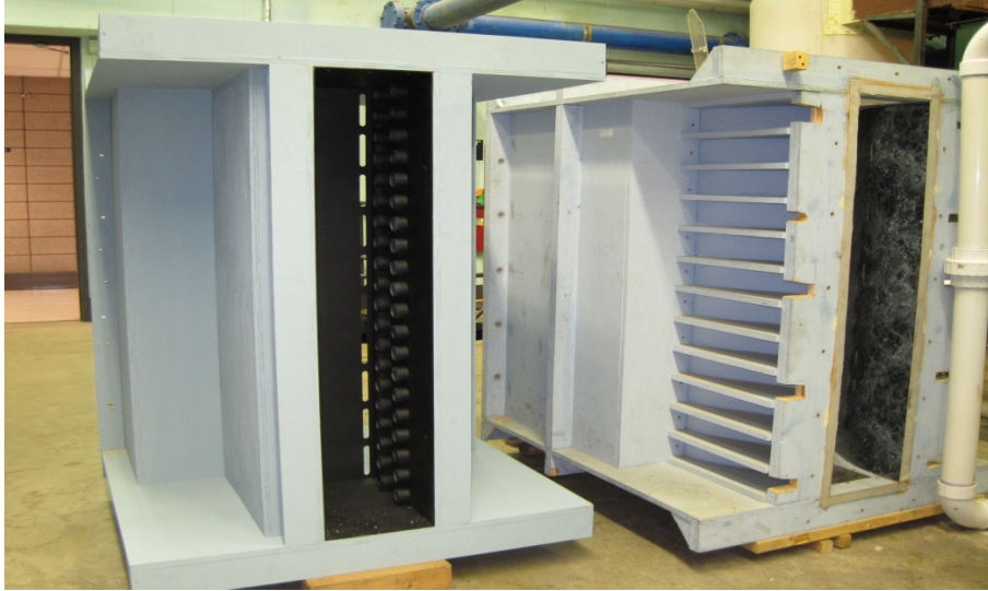
Figure 16: Front view of Aero Combustor and High Turbulence Generator.
